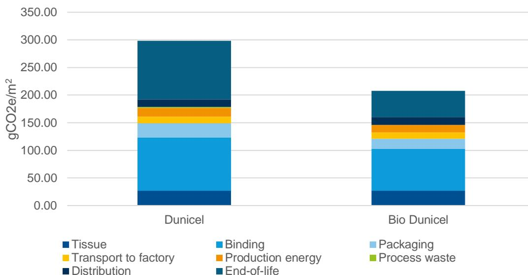
**Figure 6: Lifecycle GHG emissions comparison of Dunicel and Bio Dunicel**
